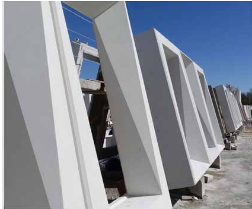
Pouring these precast punched windows for the Domino Sugar Refinery apartment complex was a large job for Gate Precast, requiring multiple concrete casts in three different profiles. Durable 3D-printed molds for concrete casting made with Big Area Additive Manufacturing (BAAM) printers have enabled the company to deliver quality precast pieces within a shorter timeline than wooden forms.
