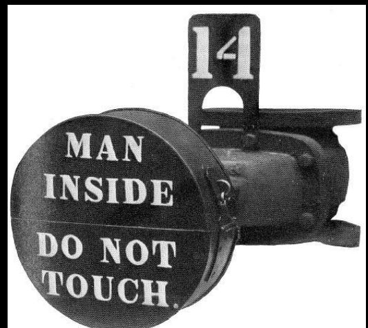
Fig. 3. Valve-Locking Device and Stencil for marking Main Steam Valve of Boiler."
