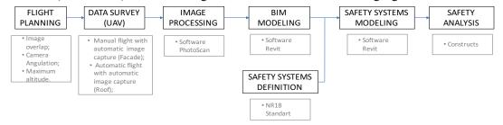
For the analysis, three constructs were considered: (a) ease of creation of the BIM model based on point cloud (registration of the facade and safety systems); (b) quality of the model (absence of visual inconsistencies and level of detail of the point cloud); and (c) applicability of models for safety perspective.
