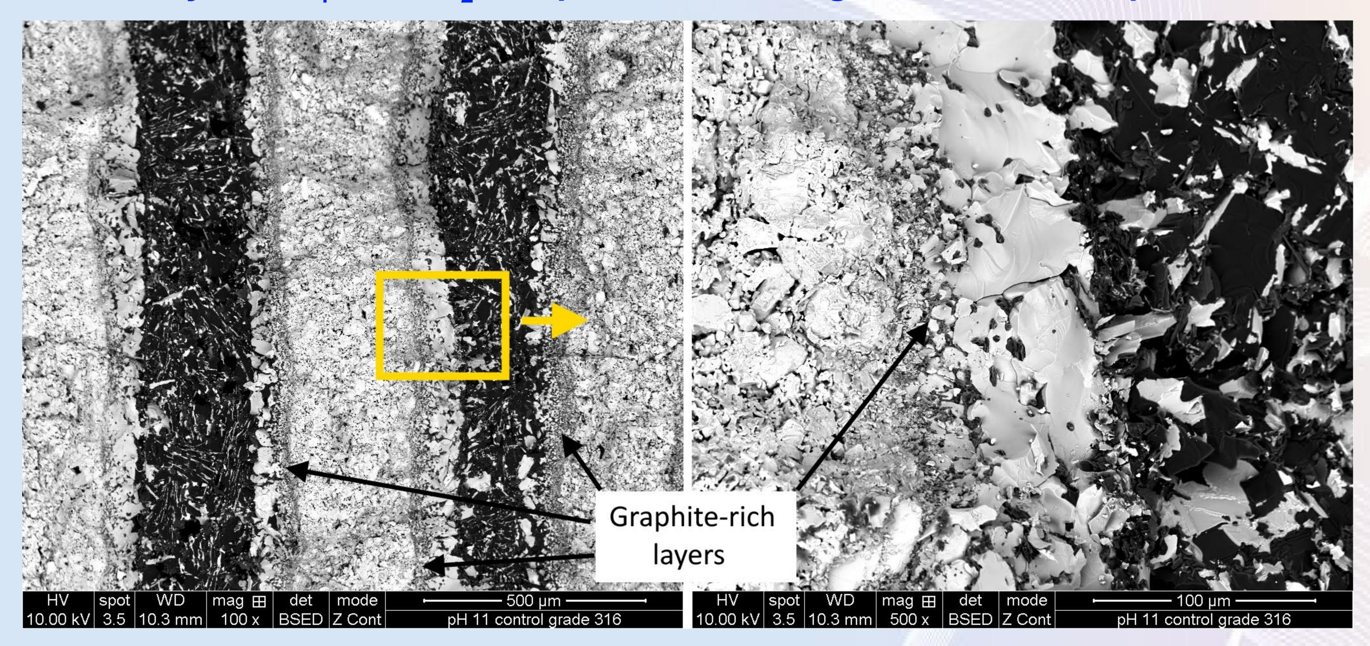
Superhard B<sub>4</sub>C and TiB<sub>2</sub> besed layers alternating with graphite-rich soft ones would provide essential bullet-proof effect with impact crack formed in the superhard layers being blunted and suppressed in the soft ones
